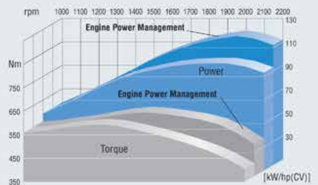
T6050 ELITE POWER & TORQUE CURVES
